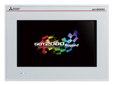
**Image 1:** With an extended operating temperature range of -20°C to +65°C, and protection rating to IP67F/IP66F, the GOT2507T-WTSD 7" operator terminal from Mitsubishi Electric meets the needs of demanding industries such as power, food and beverage and machine building.
